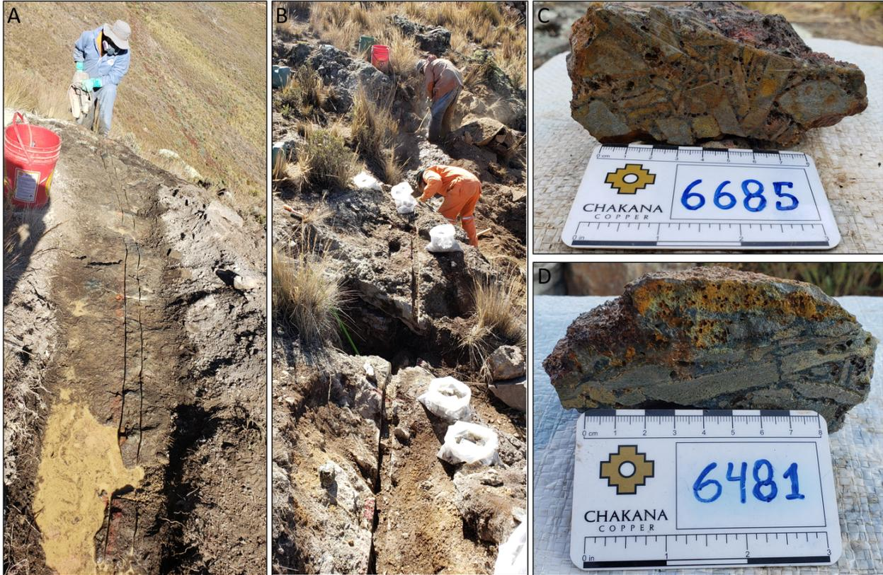
Figure 3 – photos showing channel sampling technique and examples of channel samples: A) channel cut into outcrop with diamond saw, channel width is 7.5 cm; B) channel samples are chiseled from outcrop and transferred to sample bags for each specified sample interval; C-D) examples of breccia samples from channel sampling program.
