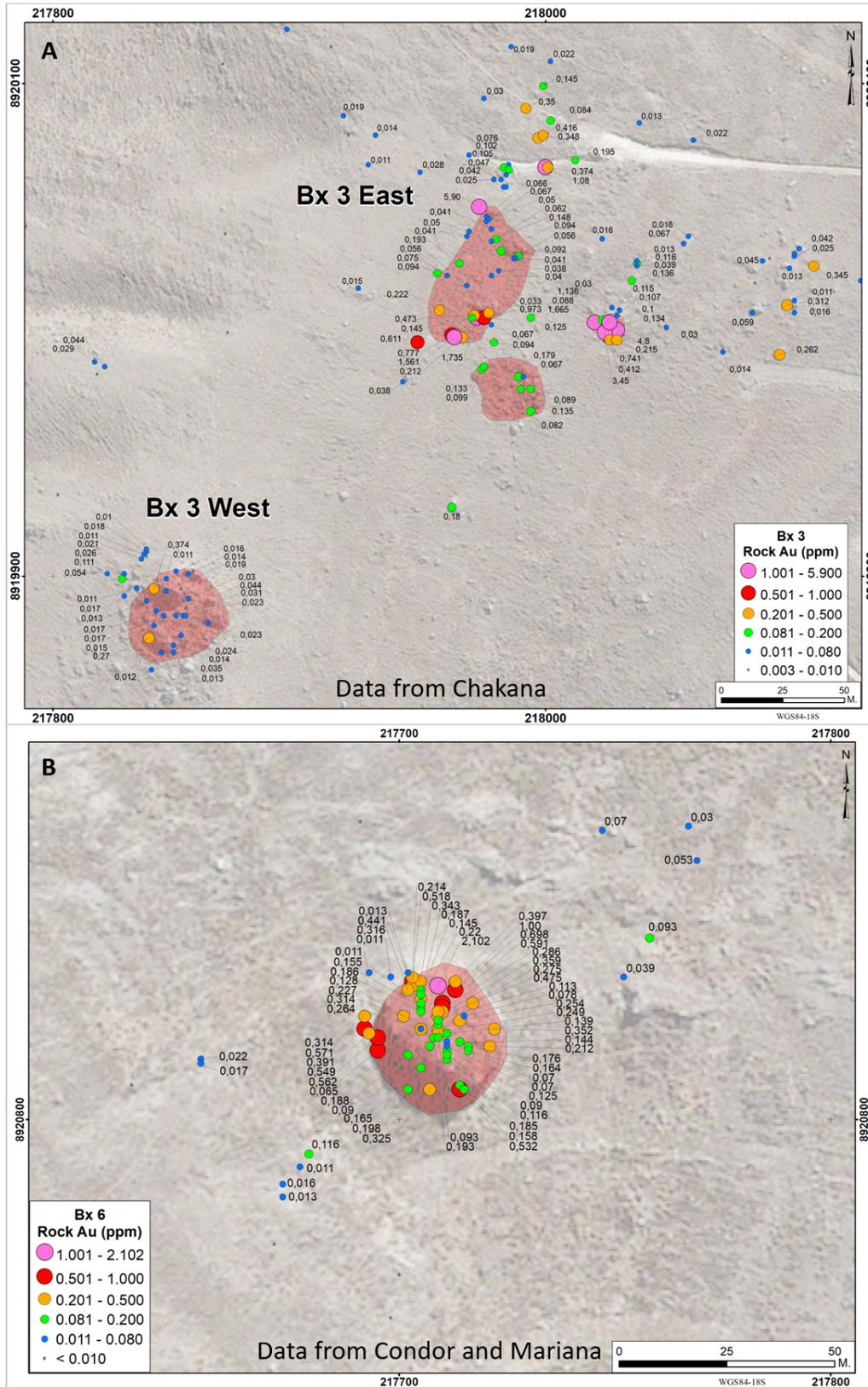
Figure 2 – Maps showing gold in surface rock samples collected by Chakana over (A) Bx 3E and Bx 3W, and samples collected by Condor Resources and Mariana Resources over (B) Bx 6. For additional results and a discussion of the sampling and analytical methods see [www.chakanacopper.com](http://www.chakanacopper.com). Readers are cautioned that surface rock samples are, by nature, selective and are unlikely to represent average grades on the Project.
