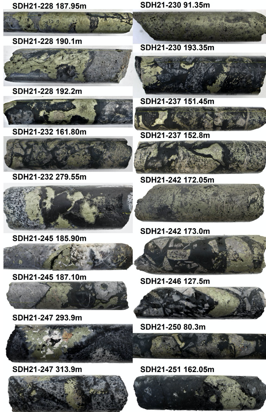
Figure 4 – Select core photos from Huancarama reported in this release: SDH21-228 (187.95m) semi-massive chalcopyrite-pyrite replacement of tourmaline breccia; SDH21-228 (190.1m) chalcopyrite filling open cavity in breccia; SDH21-228 (192.2m) chalcopyrite-tourmaline-cemented breccia; SDH21-230 (91.35m) massive chalcopyrite; SDH21-230 (193.35m) chalcopyrite-tourmaline-cemented breccia; SDH21-232 (161.80m) chalcopyrite-pyrite replacement of clasts; SDH21-232 (279.55m) chalcopyrite-tourmaline-cemented breccia; SDH21-237 (151.45m) chalcopyrite-tourmaline-cemented breccia and sulfide clast replacement; SDH21-237 (152.8m) chalcopyrite-tourmaline-cemented breccia and sulfide clast replacement; SDH21-242 (172.05m) semi-massive chalcopyrite-pyrite replacement breccia; SDH21-242 (173.0m) chalcopyrite replacement of clasts in mosaic breccia; SDH21-245 (185.9m) chalcopyrite-quartz cemented breccia; SDH21-245 (187.1m) chalcopyrite-tourmaline-cemented mosaic breccia; SDH21-246 (127.5m) chalcopyrite-tourmaline-cemented chaotic shingle breccia; SDH21-247 (293.9m) chalcopyrite-quartz-siderite-sphalerite filling cavity in breccia; SDH21-247 (313.9m) mosaic breccia with insipient granodiorite clast replacement by chalcopyrite; SDH21-250 (80.3m) chalcopyrite-tourmaline-cemented mosaic breccia and partial sulfide clast replacement; SDH21-251 (162.05m) mosaic breccia replaced by tourmaline-chalcopyrite. Core diameter is 6.35cm (HQ) in all instances.
