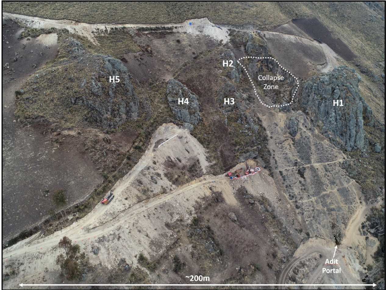
Figure 6 – Drone image looking northeast at the Huancarama Breccia Complex showing the five principal tourmaline breccia bodies exposed at surface (H1-H5), historic adit portal, and drill platforms. Note the drill rig in center of image.
