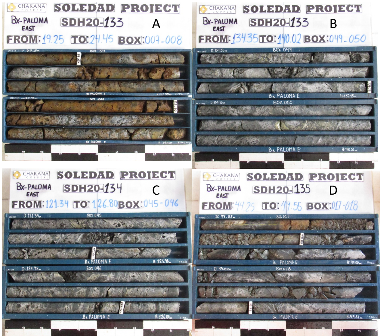
Figure 4 – Examples of mineralized core from drill holes reported in this release showing different styles of mineralization found in Paloma East: A) SDH20-133 – oxidized gold-bearing mosaic breccia with blocks of lithic tuff; the interval 19.3-24.0m assays 2.09 g/t Au and 58.3 g/t Ag; B) SDH20-133 – silicified mosaic breccia with chalcopyrite-pyrite cement; the interval 134.0-140.0m assays 0.20 g/t Au, 1.51% Cu, and 13.0 g/t Ag; C) SDH20-134 – silicified chaotic shingle breccia with quartz-chalcopyrite-pyrite cement; the interval 121.0-126.0m assays 0.16 g/t Au, 0.40% Cu, and 15.6 g/t Ag; D) SDH20-135 – contact between lithic tuff and tourmaline breccia with abundant pyrite-chalcopyrite at the margin; the interval 44.8-50.0m assays 0.51 g/t Au, 3.19% Cu, and 79.1 g/t Ag.
