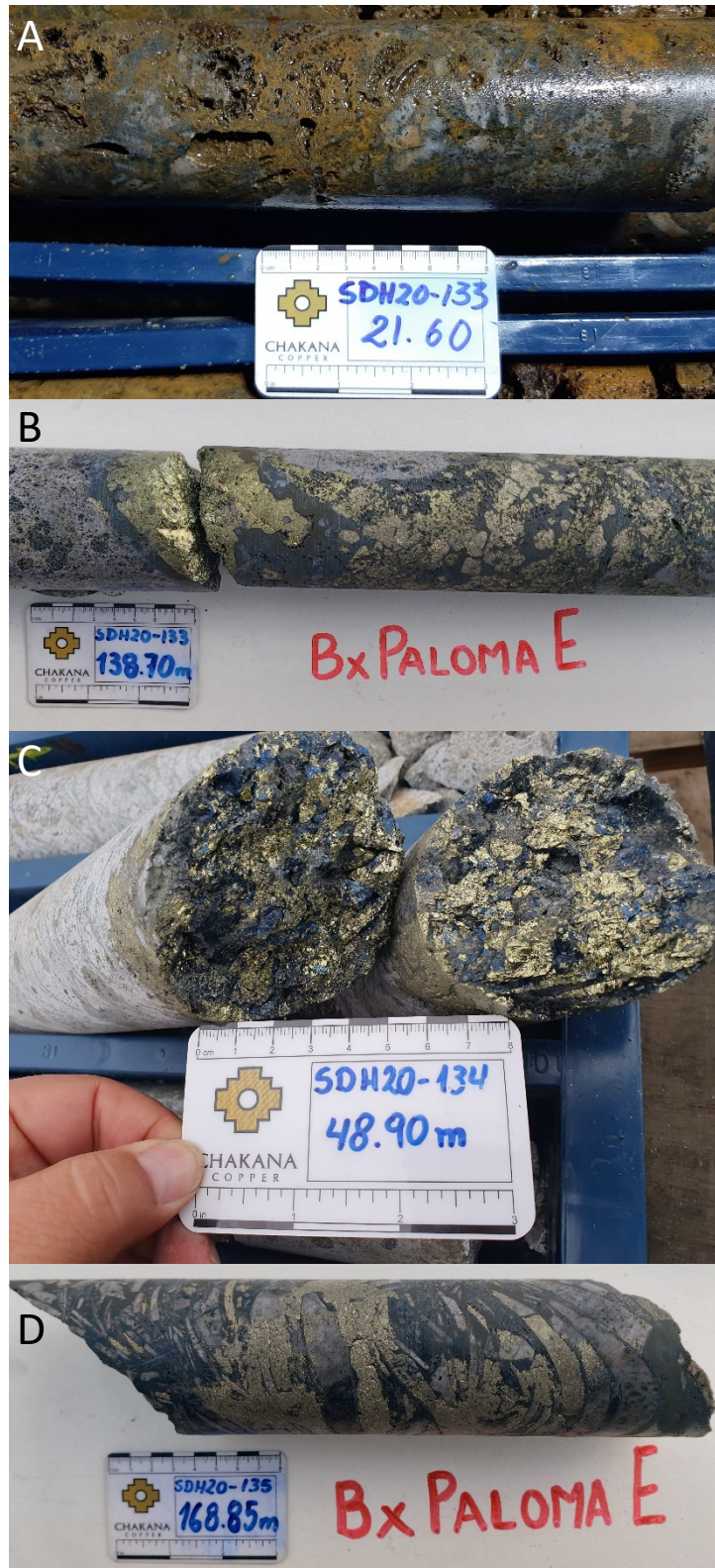
Figure 5 – Detailed core photos from Paloma East; A) SDH20-133, 21.6m, strongly oxidized gold-bearing tourmaline breccia; B) SDH20-133, 138.7m, mosaic breccia replaced by chalcopyrite-pyrite-tourmaline; C) SDH20-134, 48.9m, shingle breccia with band of massive chalcopyrite-covellite; D) SDH20-135, 168.85m, shingle breccia with tourmaline-replaced matrix and selective sulfide replacement of clasts.
