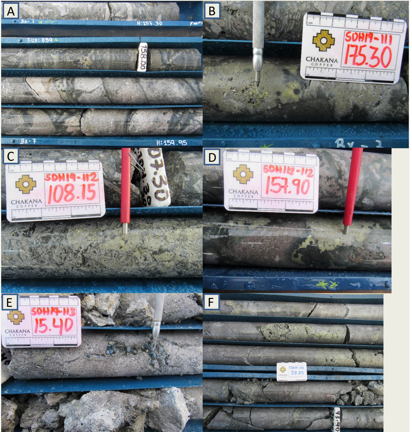
Figure 5 – Detailed core photos from drill holes discussed in this release; A) SDH19-111, 158.0m, chaotic shingle breccia and blocks with sheeted veining with quartz-pyrite-chalcopyrite cemented matrix; B) SDH11-111, 175.3m, quartz-pyrite-chalcopyrite cemented breccia; C) SDH19-112, 108.15m, mosaic breccia with tourmaline cement and chalcopyrite replacing clasts; D) SDH19-112, 157.9m, quartz-pyrite-chalcopyrite cemented breccia; E) SDH19-113, 15.4m, covellite in fracture at contact between andesite and tourmaline breccia; F) SDH19-114, 93.0m coarse mosaic breccia with pyrite-chalcopyrite cement.
