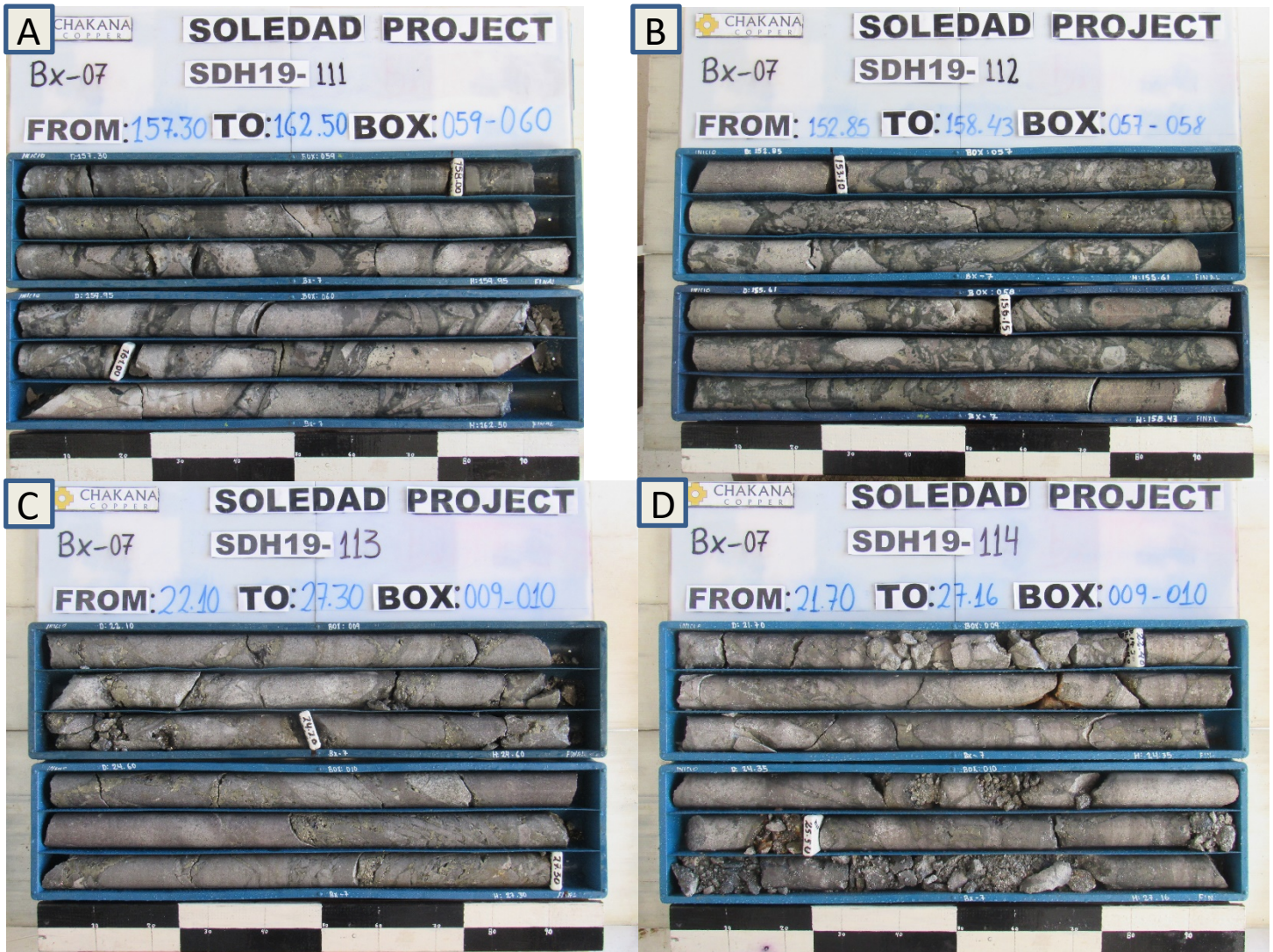
Figure 4 – Mineralized intercepts from drill holes reported in this release showing different styles of mineralization in Bx 7: A) SDH19-111 – mosaic breccia with large clasts of volcanic wall rock and quartz-sulfide cemented matrix (note vugs with euhedral quartz and sulfide minerals); the interval 157.0-163.0m assays 0.68g/t Au, 0.44% Cu, and 415.6g/t Ag; B) SDH19-112 – mosaic breccia with quartz-sulfide cemented matrix; the interval 153.0-158.0m assays 0.46g/t Au, 0.21% Cu, and 194.2g/t Ag; C) SDH19-113 – clast supported breccia with sulfide matrix (note local intervals of shingle breccia); the interval 22.0-27.0m assays 0.57g/t Au, 0.37% Cu, and 39.4g/t Ag; D) SDH19-114 – mosaic breccia with quartz-sulfide cemented matrix; the interval 22.0-27.0m assays 2.00g/t Au, 0.10% Cu, and 13.9g/t Ag.
