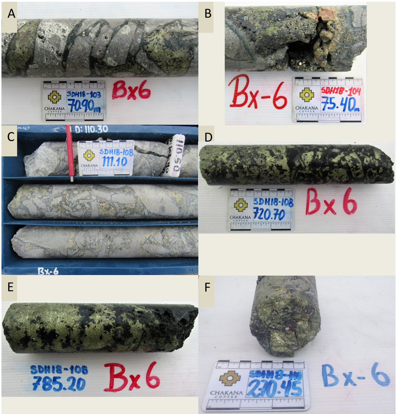
Figure 5 – Detailed core photos from drill holes discussed in this release; A) SDH18-103, 70.9m, shingle breccia with chalcopyrite-sphalerite-dominant sulfide matrix; B) SDH18-104, 75.4m, mosaic breccia with pyrite-chalcopyrite-galena-siderite matrix; C) SDH18-108, 111.1m, mosaic breccia with quartz-tourmaline-chalcopyrite-pyrite matrix; D) SDH18-108, 720.7m, tourmaline breccia with chalcopyrite-chalcocite replacement of lithic fragments; E) SDH18-108, 785.2m, tourmaline breccia with semi-massive chalcopyrite replacement; F) SDH18-110, 270.45m coarse-grained centimetre-scale chalcopyrite crystals filling matrix of tourmaline breccia.
