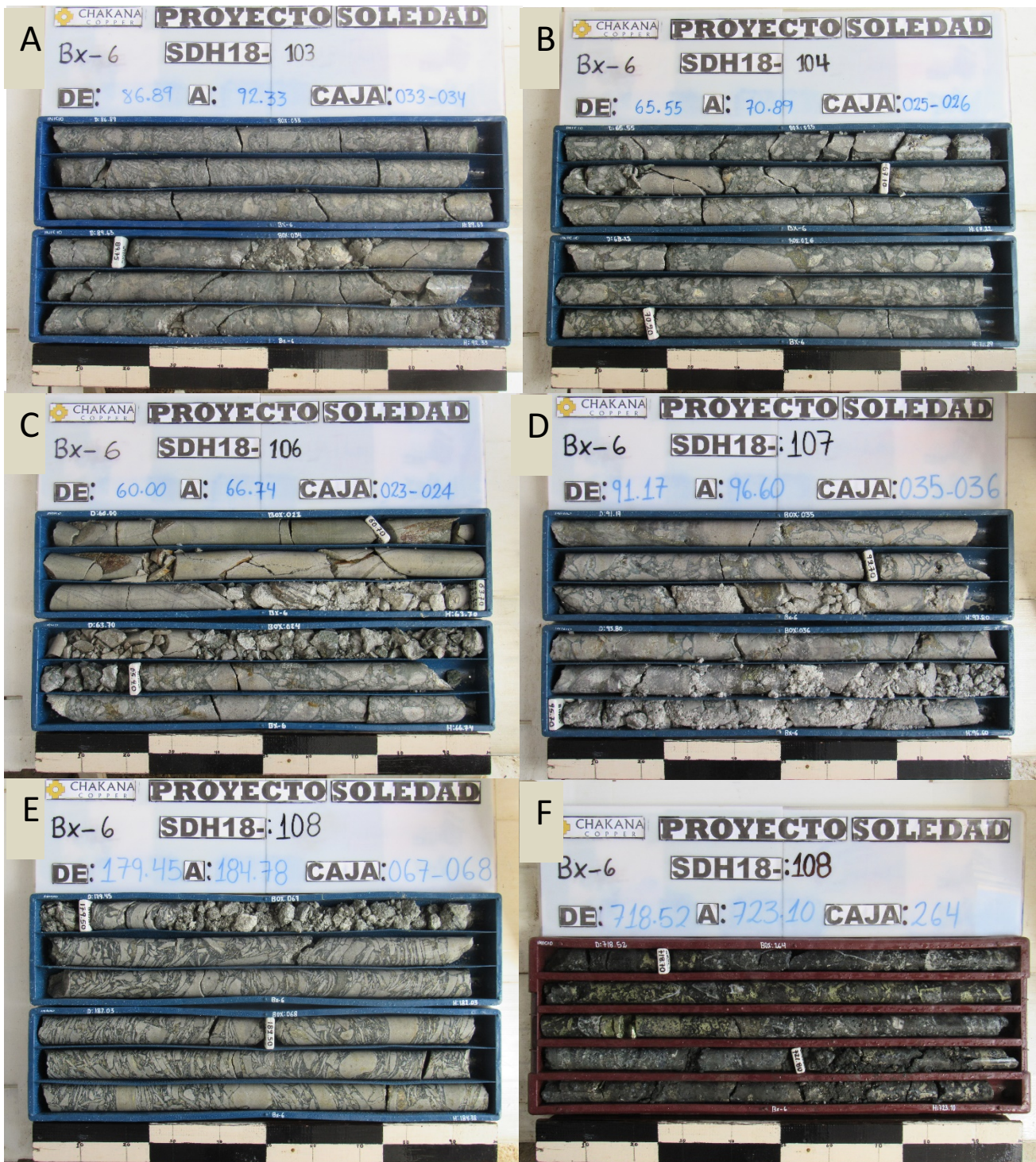
Figure 4 – Mineralized intercepts from drill holes reported in this release showing different styles of mineralization in Bx 6: A) SDH18-103 – mixed chaotic shingle and mosaic breccia with tourmaline-sulfide matrix; the interval 87.0-92.0m assays 1.49 g/t Au, 0.91% Cu, and 439.5 g/t Ag; B) SDH18-104 – mosaic breccia with tourmaline-sulfide matrix; the interval 66.0-71.0m assays 0.80 g/t Au, 1.20% Cu, and 470.8 g/t Ag; C) SDH18-106 – contact between wallrock and mosaic breccia; the interval 62.1-67.0m assays 1.17 g/t Au, 0.63% Cu, and 467.0 g/t Ag; D) SDH18-107 – mosaic breccia with tourmaline-sulfide matrix; the interval 91.0-96.0m assays 2.62 g/t Au, 2.81% Cu, and 722.6 g/t Ag; E) SDH18-108 – shingle breccia with tourmaline-sulfide matrix; the interval 179.0-185.0m assays 4.93 g/t Au, 0.26% Cu, and 168.3 g/t Ag; F) SDH18-108 – tourmaline breccia with intense sulfide replacement; the interval 718.0-723.0m assays 0.43 g/t Au, 3.69% Cu, and 16.5 g/t Ag.
