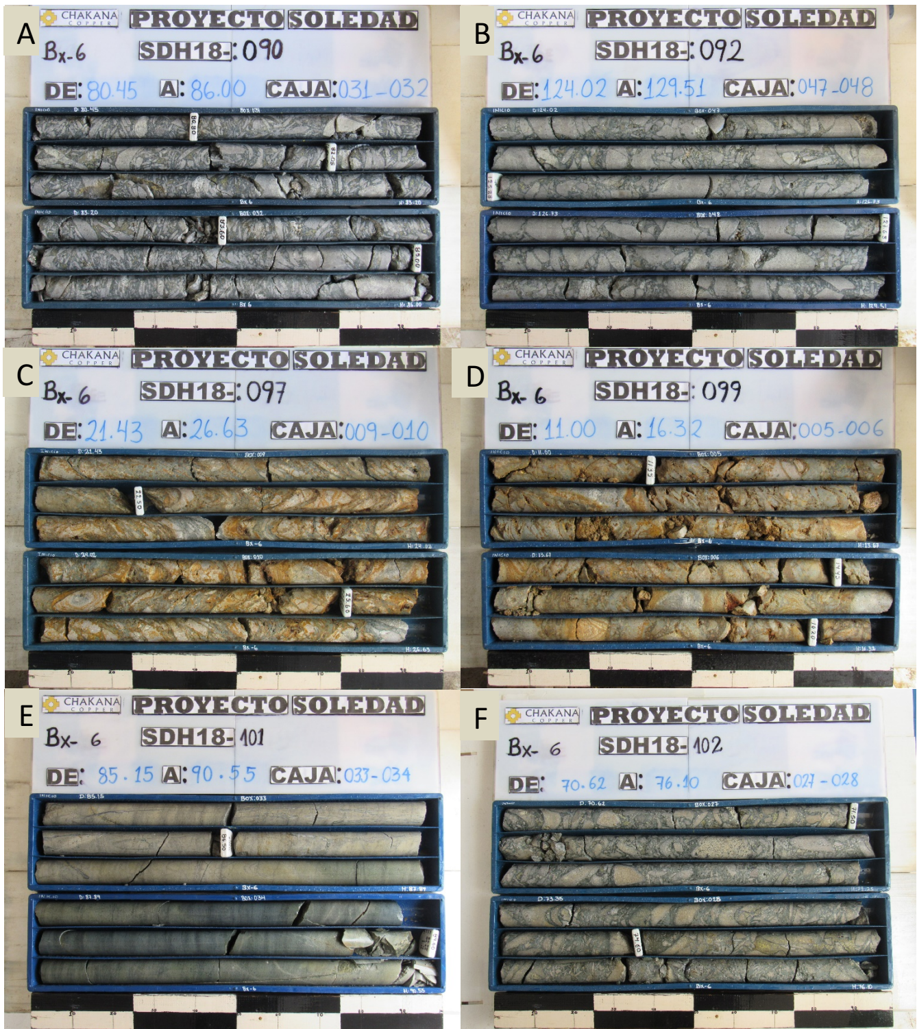
Figure 4 – Mineralized intercepts from drill holes reported in this release showing different styles of mineralization in Bx 6: A) SDH18-090 – chaotic shingle breccia with tourmaline-sulfide matrix; the interval 80.0-86.0m assays 1.77 g/t Au, 0.97% Cu, and 240.7 g/t Ag; B) SDH18-092 – mosaic breccia with tourmaline-sulfide matrix; the interval 124.0-129.0m assays 0.80 g/t Au, 0.36% Cu, and 249.8 g/t Ag; C) SDH18-097 – oxidized shingle breccia; the interval 21.0-26.0m assays 1.01 g/t Au, 0.04% Cu, and 140.8 g/t Ag; D) SDH18-099 – oxidized mosaic breccia with variable clast sizes; the interval 11.0-16.0m assays 0.77 g/t Au, 0.05% Cu, and 161.8 g/t Ag; E) SDH18-101 – sheeted quartz-tourmaline-sulfide veining in porphyritic andesite host rock; the interval 85.0-89.50m assays 6.59 g/t Au, 0.02% Cu, and 71.8 g/t Ag; F) SDH18-102 – mixed mosaic and chaotic shingle breccia with tourmaline-sulfide matrix; the interval 71.0-76.0m assays 2.07 g/t Au, 1.95% Cu, and 3,023.0 g/t Ag.
