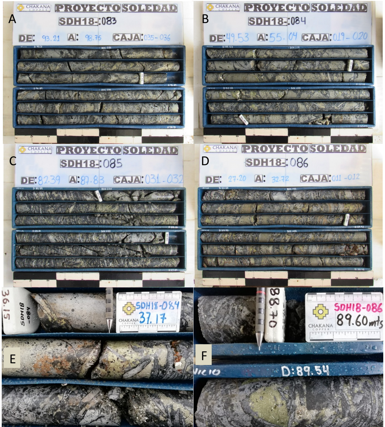
Figure 3 – Mineralized intercepts from drill holes reported in this release showing different styles of mineralization in Bx 5: A) SDH18-083 – shingle breccia with strong tourmaline replacement; the interval 93.85-99m assays 1.79 g/t Au, 0.42% Cu, and 24.1 g/t Ag; B) SDH18-084 – chaotic shingle and mosaic breccia; the interval 49-55m assays 0.49 g/t Au, 1.77% Cu, and 18.86 g/t Ag; C) SDH18-085 – shingle breccia with strong tourmaline replacement; the interval 82-88m assays 0.42 g/t Au, 2.13% Cu, and 27.6 g/t Ag; D) SDH18-086 – shingle breccia with variable clast sizes; the interval 27-33m assays 1.24 g/t Au, 1.43% Cu, and 59.9 g/t Ag; E) breccia with interstitial chalcopyrite and pyrite in SDH18-084 at 37.17m; F) chalcopyrite and pyrite filling open space in shingle breccia; SDH18-086 at 89.6m.
