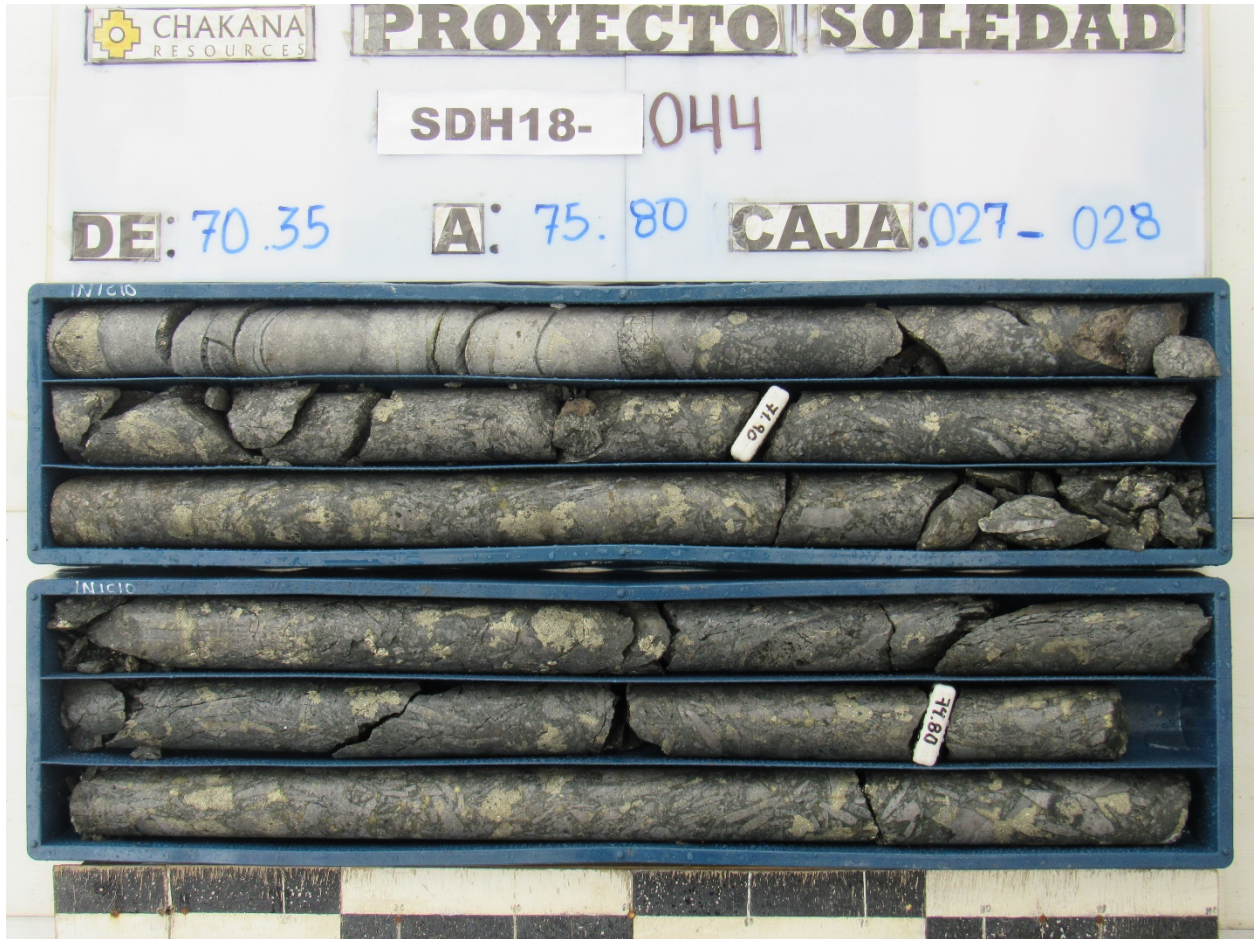
Figure 1 – High grade margin zone mineralization from hole SDG18-044 in Bx 1. The six metre interval from 70.0-76.0 averages 2.76% Cu, 8.33 g/t Au, and 19.6 g/t Ag.
