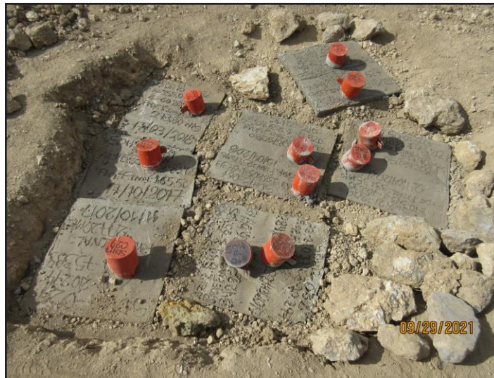
Figure 12.1: Breccia 1 Drill Pad with Several Drill Collars
