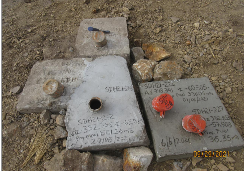
Figure 10.1: Permanent Cement Drill Collar Markers
