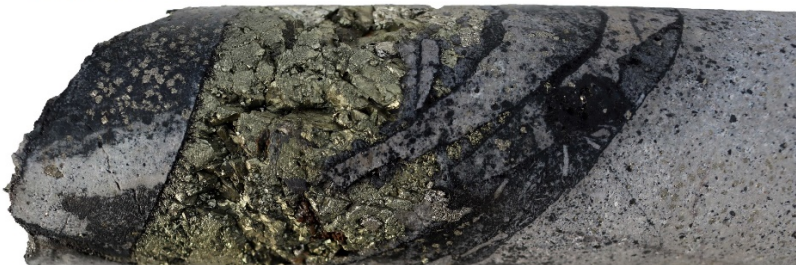
Figure 4 – Select core photos from Bx 5 reported in this release: SDH21-244 (34.7m) shingle breccia cemented with chalcopyrite-pyrite; SDH21-252 (33.9m) chaotic shingle breccia with chalcopyrite-pyrite in matrix; SDH21-253 (41.5m) chaotic shingle breccia with chalcopyrite-pyrite in matrix; SDH21-255 (39.6m) shingle breccia cemented with chalcopyrite-pyrite; SDH21-256 (110.55m) chaotic shingle breccia with semi-massive chalcopyrite-pyrite; SDH21-258 (35.45m) shingle breccia cemented with chalcopyrite-pyrite; SDH21-261 (39.25m) chaotic shingle breccia with semi-massive chalcopyrite-pyrite. Core diameter is 6.35cm (HQ) in all instances.
