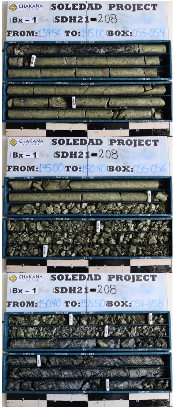
Figure 4 – Massive sulfide intersected in the North Zone breccia pipe at Bx 1. Core diameter is 6.35cm (HQ).
