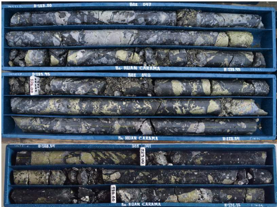
Figure 4 – Core photos from Huancarama: SDH20-163 (83.3m) mosaic tourmaline breccia with partial clast replacement by chalcopyrite; SDH20-163 (117.85m) tourmaline breccia with chalcopyrite and red sphalerite open space filling ; SDH20-164 (123.2 to 131.12m) - example of high-grade copper sulfide (chalcopyrite) clast replacement and sulfide-cemented breccia. Core diameter is 6.35cm (HQ) in all instances.
