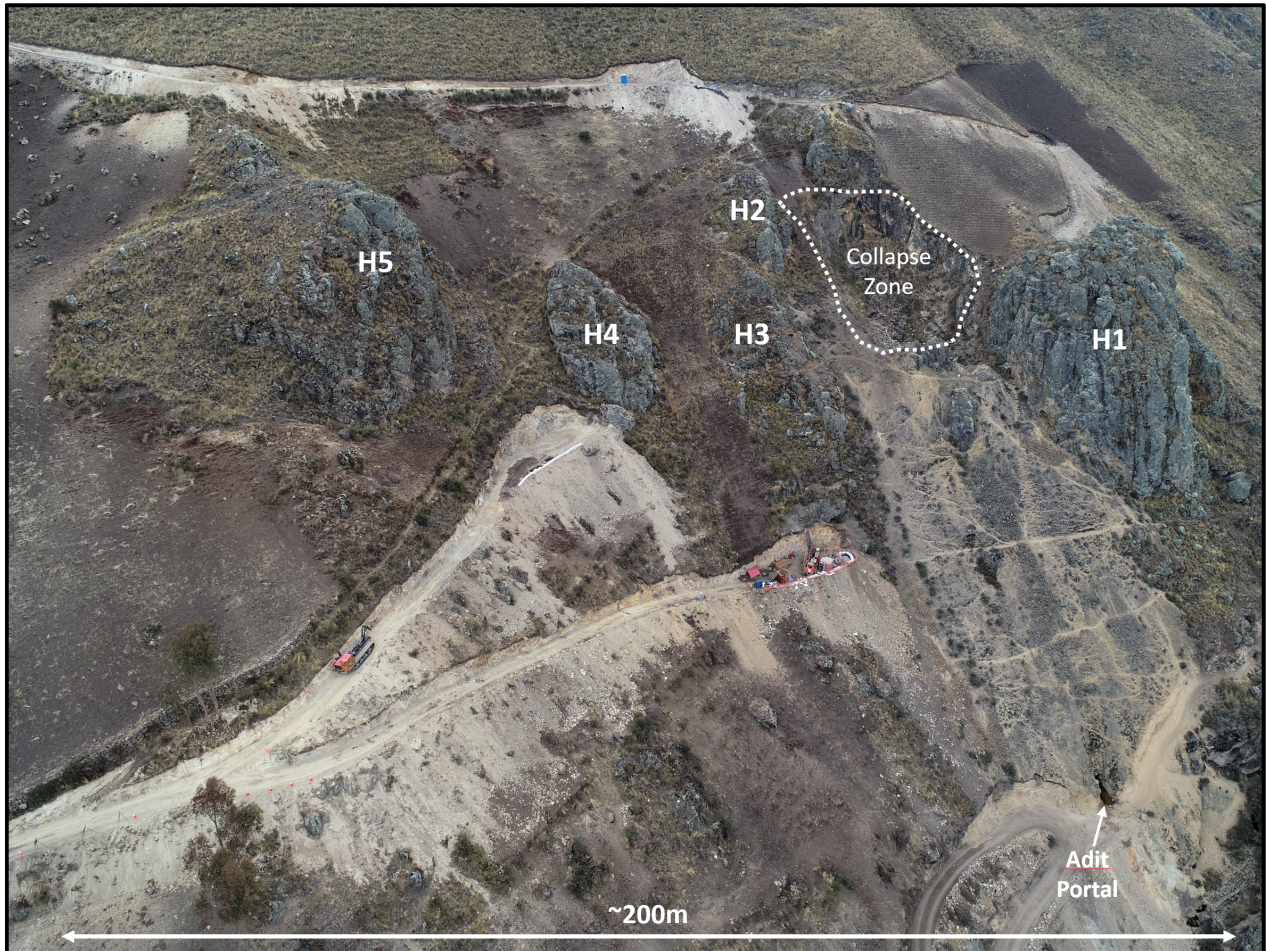
Figure 5 – Drone image looking northeast at the Huancarama Breccia Complex showing the five principal tourmaline breccia bodies exposed at surface (H1-H5), historic adit portal, and drill platforms. Note drill rig in center of image.
