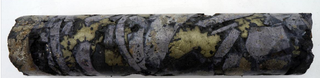
Figure 4 – Detailed core photos from Paloma West: SDH20-150 (79.4m) quartz-chalcopyrite-pyrite-tourmaline cemented breccia; SDH20-151 (46.6m) mosaic breccia replaced by chalcopyrite-pyrite; SDH20-151 (89.3m) mosaic breccia with chalcopyrite-pyrite cement and late euhedral pyrite replacement; SDH20-152 (34.85m) chaotic shingle breccia with chalcopyrite-pyrite cement; F) SDH20-152 (41.9m) shingle breccia with chalcopyrite-pyrite cement.
