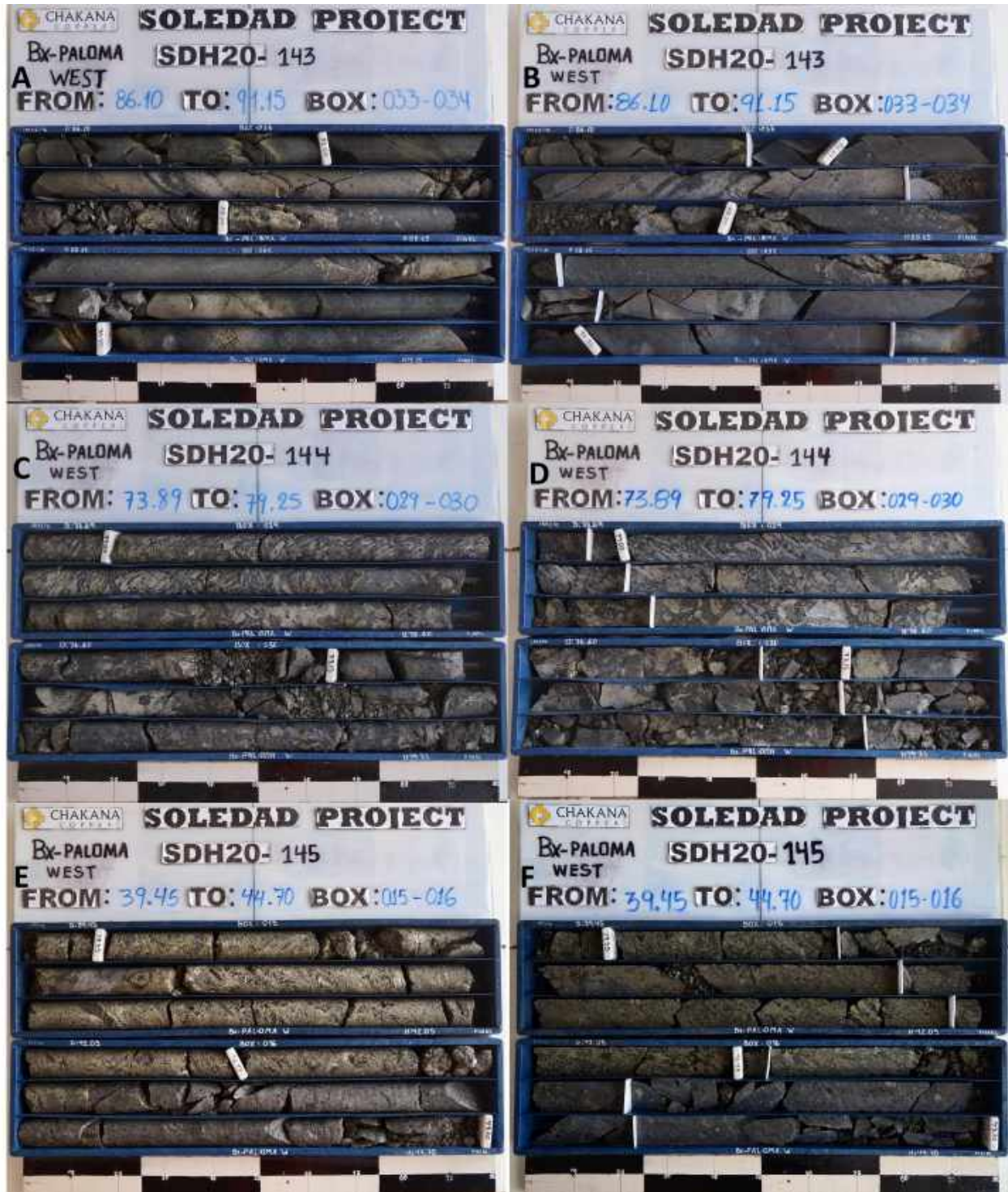
Figure 6 – Examples of mineralized core from drill holes reported in this release showing different styles of mineralization found in Paloma West: A) SDH20-143 – tourmaline-sulfide replacement structure; the interval 87.7-89.7m assays 11.93 g/t Au, 3.88% Cu, and 137.3 g/t Ag; B) SDH20-143 – same as A) cut core after sampling; C) SDH20-144 – chaotic shingle breccia with abundant chalcopyrite-pyrite transitioning into mosaic breccia; the interval 73-79m assays 0.91 g/t Au, 0.81% Cu, and 27.6 g/t Ag; D) SDH20-144 – same as C) cut core after sampling; E) SDH20-145 – sulfide-replaced chaotic shingle breccia with abundant chalcopyrite-pyrite; the interval 39-43.1m assays 7.20 g/t Au, 12.42% Cu, and 163.2 g/t Ag; F) SDH20-145 – same as E) cut core after sampling.
