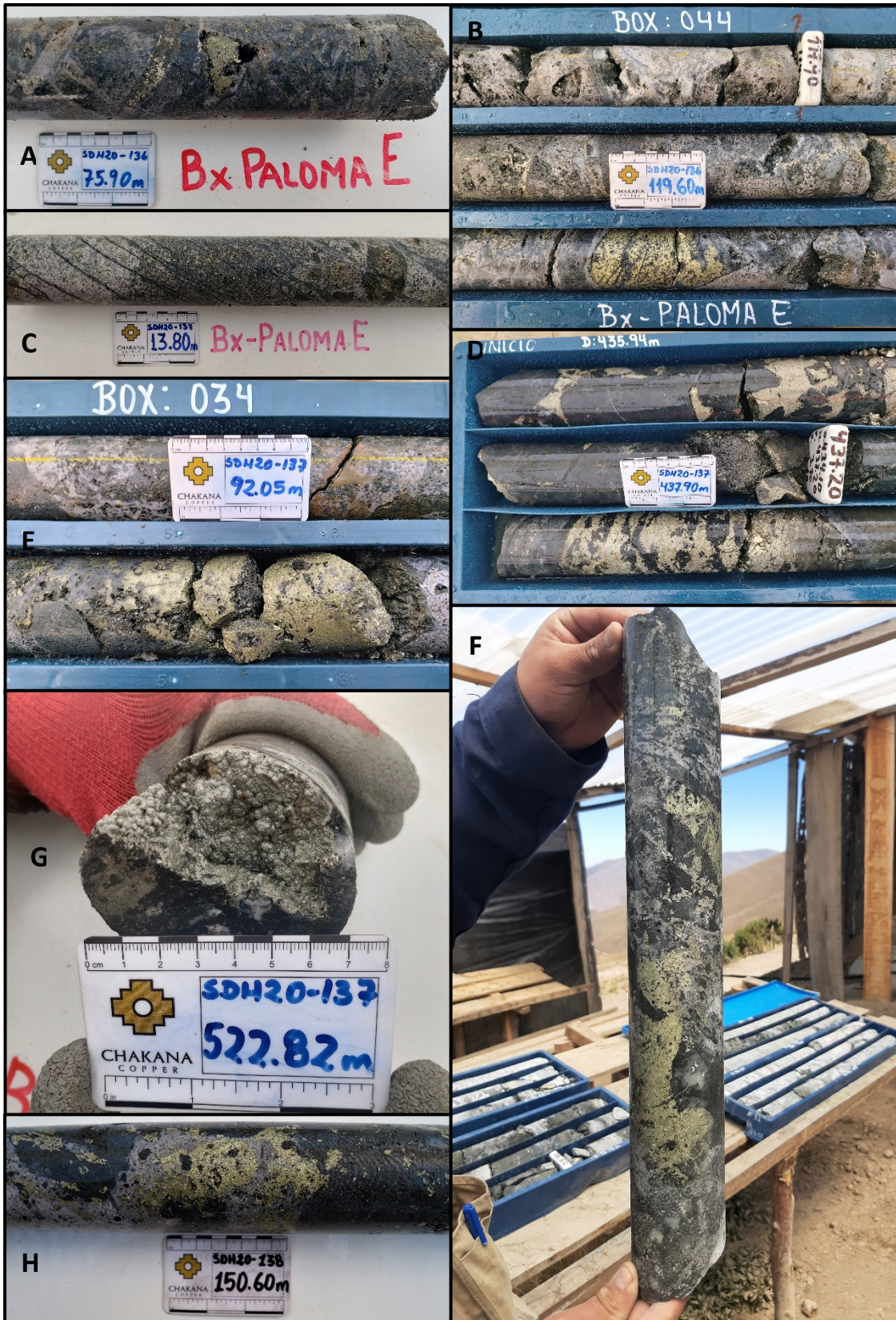
Figure 6 – Detailed core photos from Paloma East: A) SDH20-136 (75.9m) chaotic shingle breccia with chalcopyrite filling vug; B) SDH20-136 (119.6m) silicified mosaic breccia with clast replaced by chalcopyrite; C) SDH20-137 (13.8m) sheeted veining in andesitic tuff wallrock adjacent to breccia; D) SDH20-137 (437.9m) pyrite-cemented tourmaline mosaic breccia; E) SDH20-137 (92.05m) chalcopyrite replacement in silicified mosaic breccia; F) SDH20-137 (149.8m) mosaic breccia with late chalcopyrite replacement; G) SDH20-137 (522.82m) botryoidal pyrite; H) SDH20-138 (150.6m) mosaic breccia with late chalcopyrite replacement.
