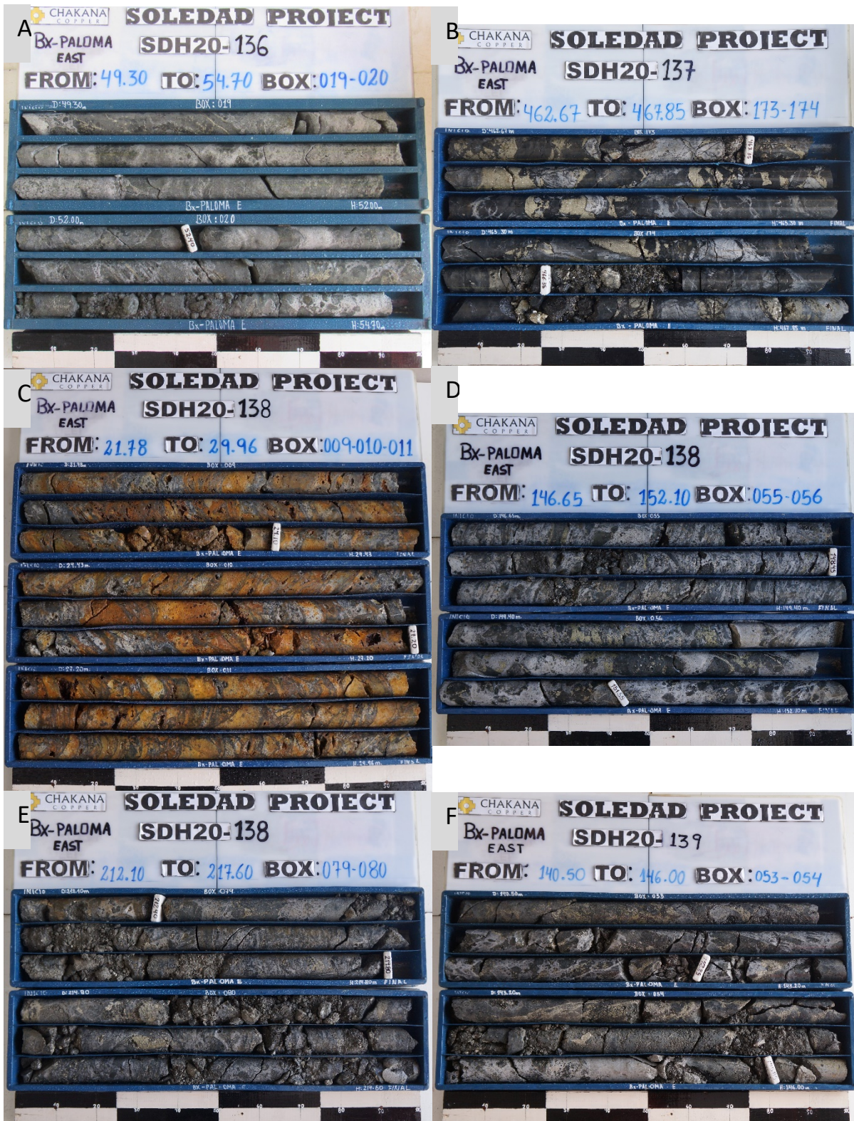
Figure 5 – Examples of mineralized core from drill holes reported in this release showing different styles of mineralization found in Paloma East: A) SDH20-136 – mosaic breccia; the interval 49.35-55.70m assays 0.16 g/t Au, 2.27% Cu, and 37.6 g/t Ag; B) SDH20-137 – tourmaline mosaic breccia with pyrite matrix; C) SDH20-138 – oxidized shingle breccia; the interval 21.00-30.00m assays 2.50 g/t Au and 18.0 g/t Ag; D) SDH20-138 – shingle and mosaic breccia; the interval 147.0-153.0m assays 0.15 g/t Au, 1.15% Cu, and 17.0 g/t Ag; E) SDH20-138 – mosaic breccia; the interval 212.0-217.0m assays 0.33 g/t Au, 0.64% Cu, and 139.5 g/t Ag; F) SDH20-139 – mosaic breccia; the interval 140.0-145.9m assays 0.53 g/t Au, 1.28% Cu, and 107.3 g/t Ag.
